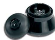
6 x 50ml rotor 21,000 rpm / 41,410 xg
